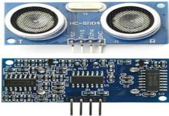
Figure 3: Ultrasonic Sensor
