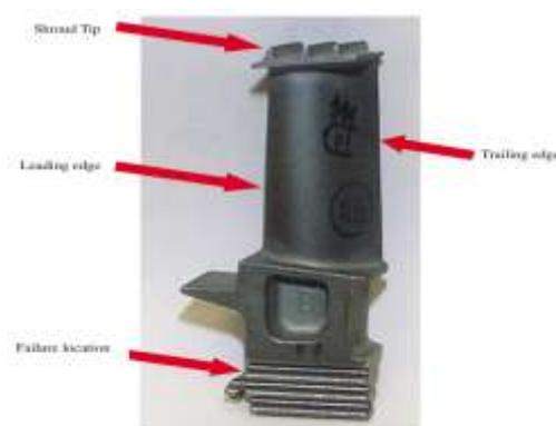
Fig1. Blade failure location
