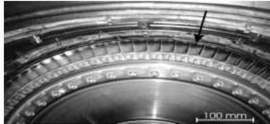
Fig6: Uneven clearance between blade tip and rotor lining
