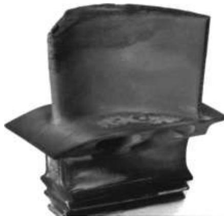
Fig2: View of a failed blade
