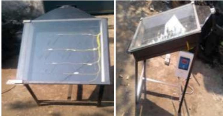
Fig 2: Actual Setup of Solar air heater with roughness on Absorber plate
