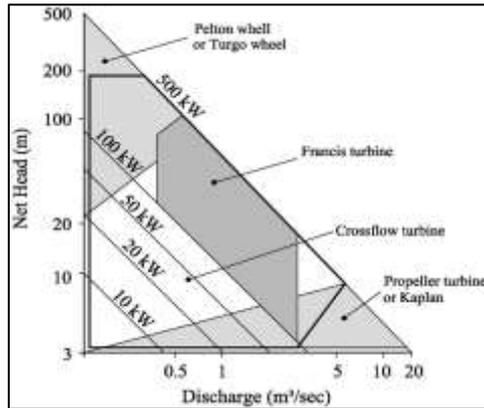
Fig.2 Turbine selection according to net head and discharge
