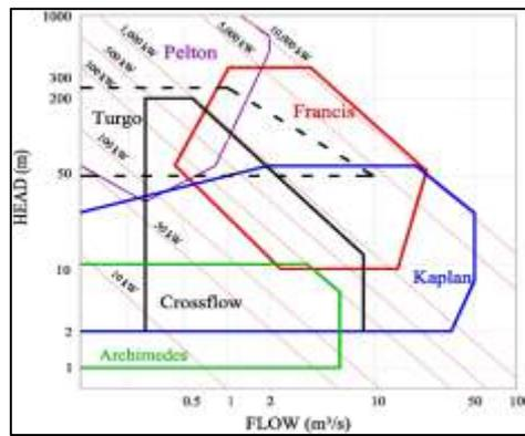
Fig.3 Turbine selection according to net head and flow rate
