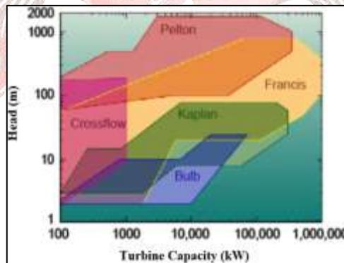
Fig.4 turbine selection according to head and turbine capacity
