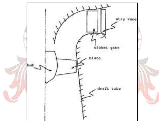
Fig.10 Blade and casing arrangement in a Kaplan turbine.[5]
