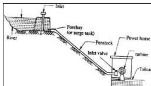
Fig.1 Schematic of a Micro Hydro Power Plant.
