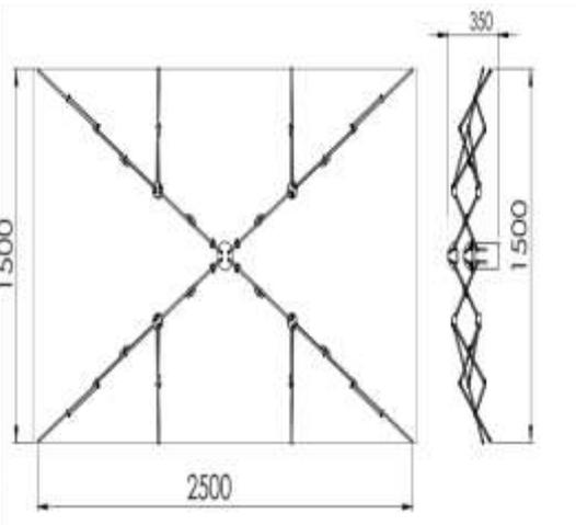
Fig. 2.Linkages engineering drawing
