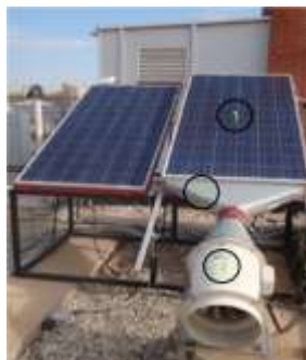
Fig. 5. Hybrid solar Photovoltaic/Thermal system cooled by forced air circulation [33].
