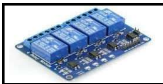
Figure: 6 Relay Board.
