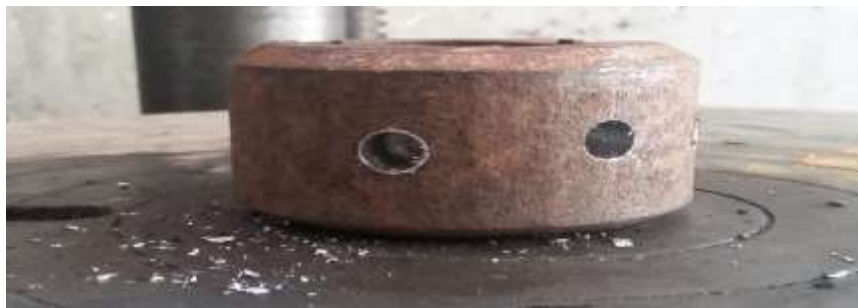
Shows drilled hole on workpiece for setup of 30° angle.
