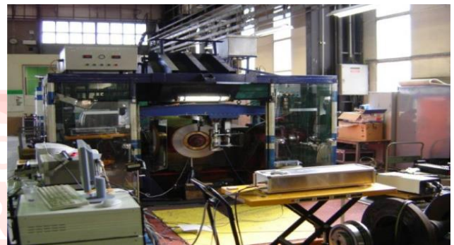
Fig 17:-Experimental Setup of Laser Scanning Vibrometer
