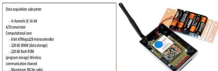
Fig. 1: Hardware profile of wireless modular monitoring system (WiMMS)
