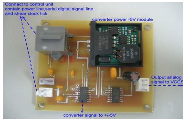
Fig. 8: On board that convert the 16bit digital voltage to analog signal with 0.~1.0 Volt.
