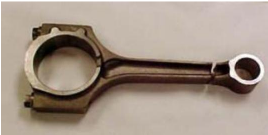
Figure 1 : Failure of a connecting rod
