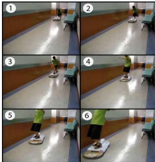
Fig.5 Sequential pictures showing the Hoverboard gliding on air while transporting a person weighing ~60Kg
