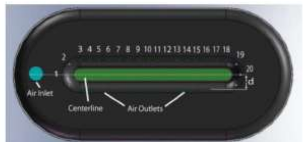
Fig.8 Geometric considerations for the fluid dynamic simulation model.
