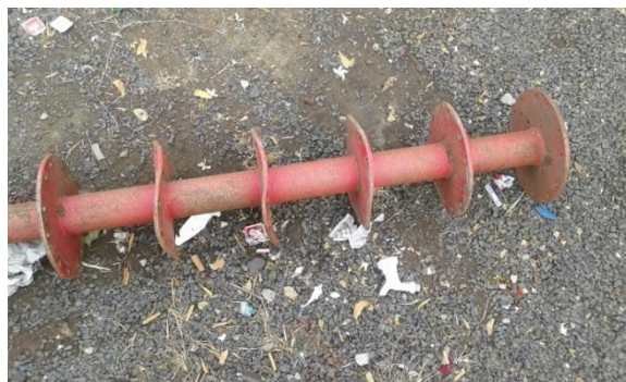
Fig.2 Failure of Rotor Shaft (Flange)
