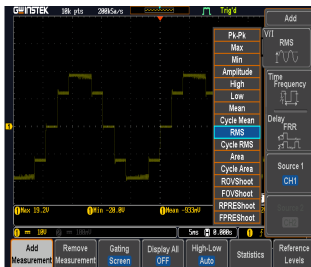
Fig.6 Experimental result of of five level cascaded H-bridge multilevel inverter
