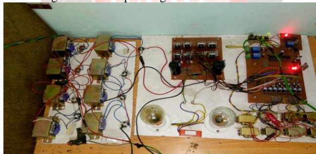
Fig. 5 Experimental setup of five level cascaded H-bridge multilevel inverter
