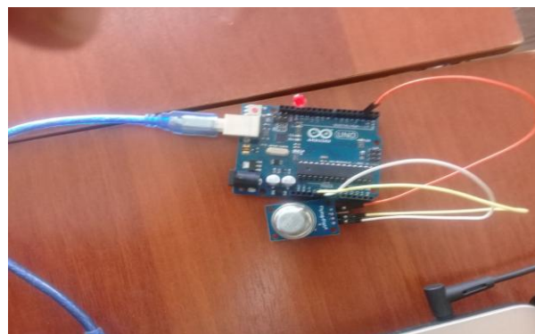
Pic 3. Connecting the MQ-2 sensor to an Arduino Uno Arduino UNO programming code
