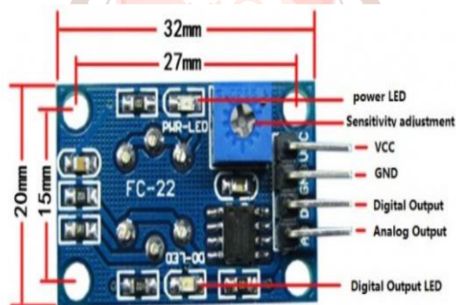
Pic 2. Microprocessor control side of MQ-2 sensor
