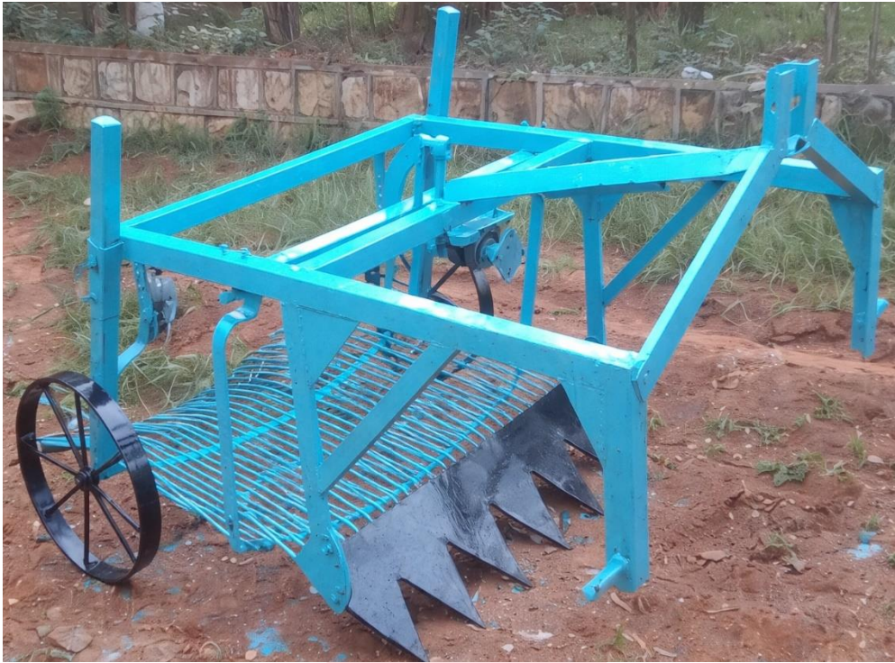
Figure 11: Designed and manufactured carrot digger
