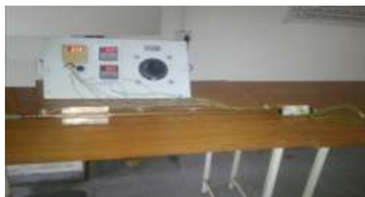
Fig: 1.2 Heat Pipe under study with control panel
